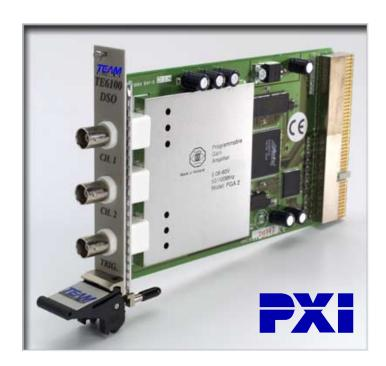
The TE6100 is the first 100 MS/SEC measuring instrument that consists of a Digital Storage Oscilloscope, Spectrum Analyzer, Transient recorder and Voltmeter. This new PXI based, compact measuring instrument, can solve almost every measurement problem. Analyzing signals is done with an 8-bit resolution and a maximum sampling speed of 100 MHz. The input ranges 0.1 Volt full scale to 80 Volt full scale. The record length is 32K/64K samples.
